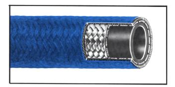
The braided polyester outer cover over AE701 hose adds minimal weight and provides superior chafe resistance. Flexibility is not impaired, and the increase in O.D. is less than .100" for all sizes. For more information on AE701 hose, ask for AEB-230. It explains how the size and complexity of hose inventory can be reduced because of hose compatibility with nearly all fluids.
